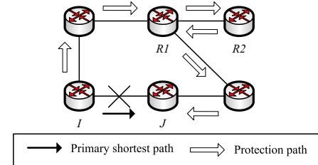
Fig. 1. Protecting link  $I-J$  using  $R2$  as a tunnel endpoint
