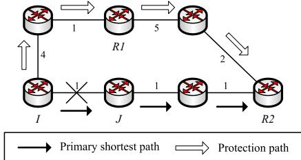
Fig. 2. Delivering packets to  $R_2$  using  $R_1$  when link  $I-J$  fails
